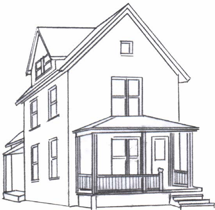
Figure 14. Dormer style alters the character of the house. Gable above matches the original roofline. Shed dormer below gives a different look.
